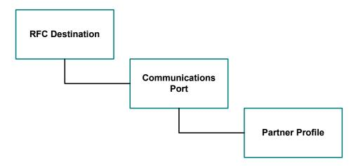
The RFC Destination defines the entity to which Remote Function Calls (RFCs) can be made; it is the same as the Logical System in the Distribution Model. The Communications Port defines a channel for communication of IDocs. The Partner Profile acts as an identifier for the eGate system, and provides a communications gateway by incorporating elements of the ALE interface.
